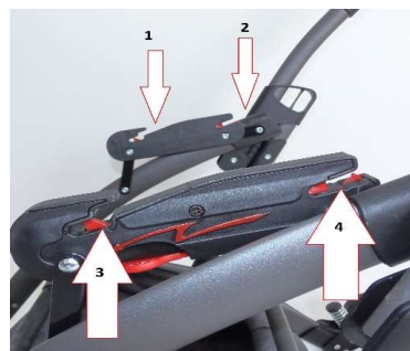
Fig. 10.1.1 Hooks for mounting the seat
